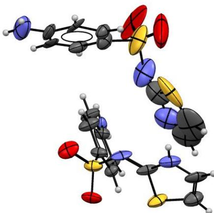
Figure 2 – Sulfathiazole form I at 34 kbar with probability ellipsoids drawn at the 50% level
