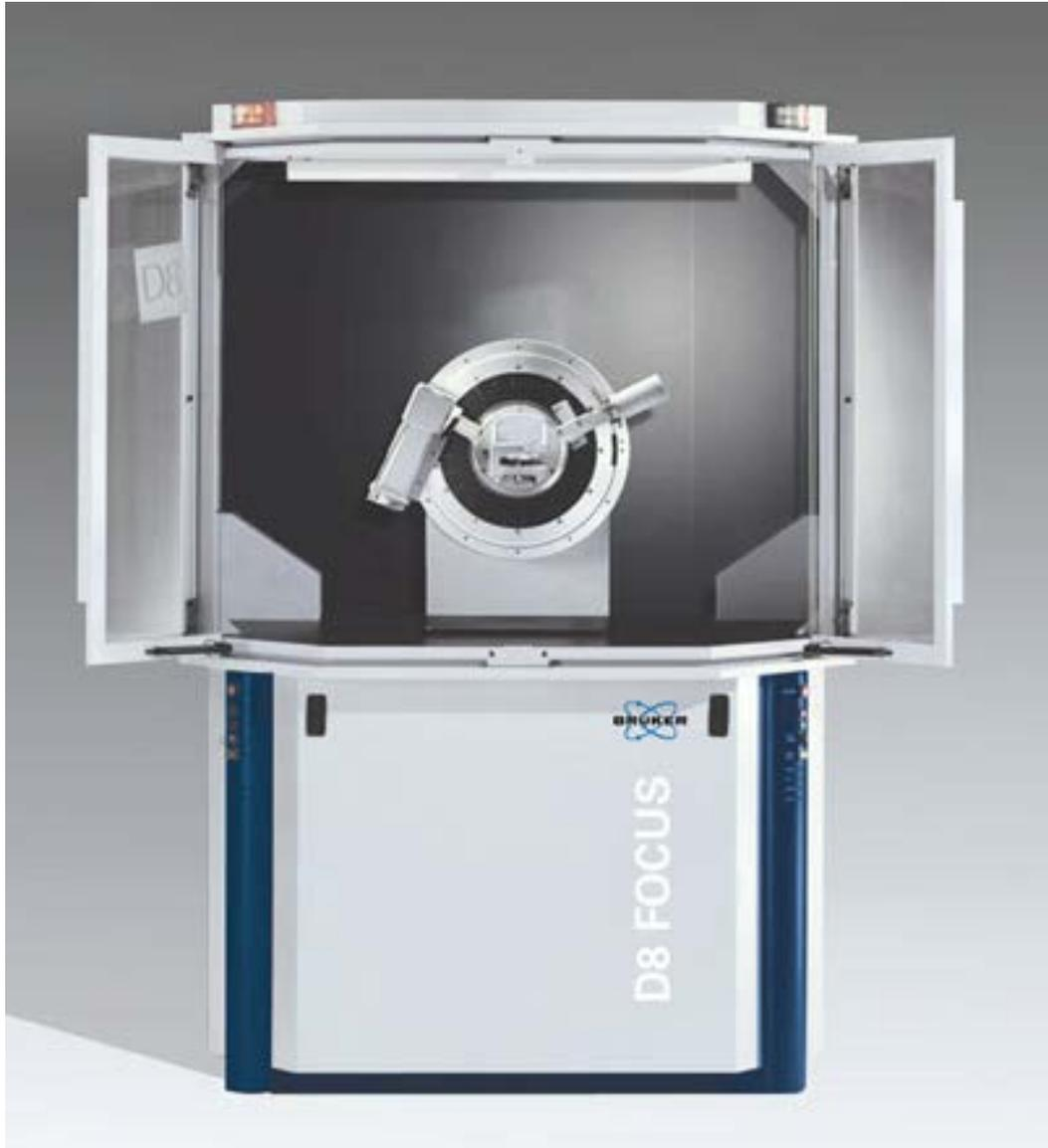
In this diffractometer with Bragg-Brentano geometry, the sample is stationary, and the counter and X-ray source are moved so that they make the same angle with the plane of the sample.
