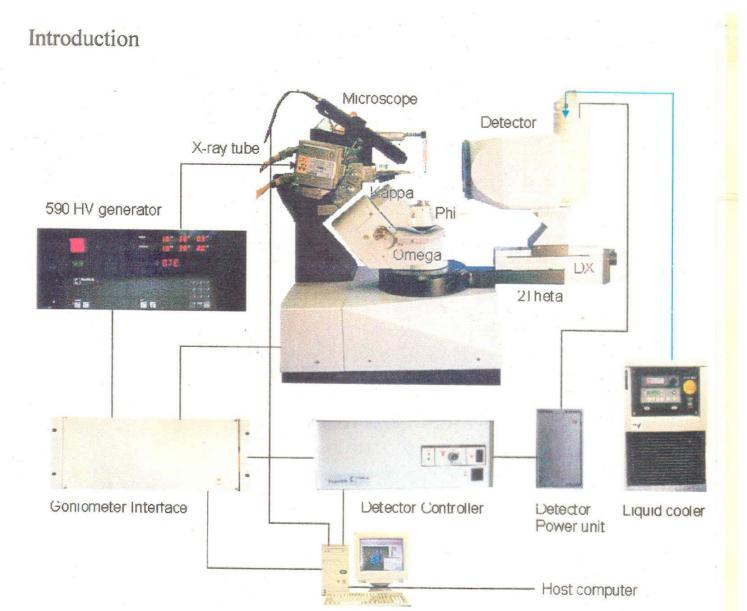
The KappaCCD consists of a X-ray source, 3-axes goniometer (Omega, Kappa, Phi) to position the crystal and a Theta-axis and DX to position the detector. The two-dimensional detector measures the X-ray, which is reflected in
