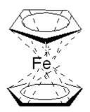
• Like some of the above acyclic organometallic ligands, the atoms of the C<sub>5</sub>H<sub>5</sub><sup>-</sup> ligand are essentially planar. The ferrocene iron ion is situated between two parallel C<sub>5</sub>H<sub>5</sub><sup>-</sup> ligands, halfway between the two rings and along the perpendicular connecting the ring centroids. These features are highlighted below, and are more clearly illustrated when you manipulate *FEROCE27* in the 3D viewer.
